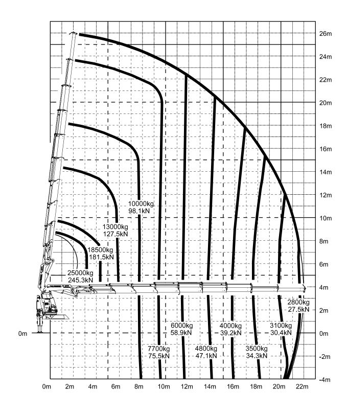
When using mechanical boom extensions, the loads shown on the charts need to be reduced by the weight of these extensions.
